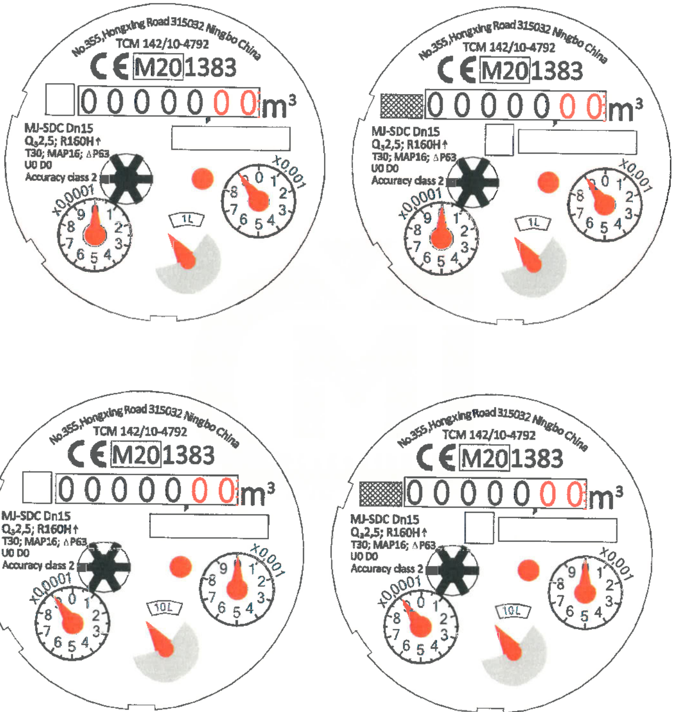
Figure 23: Examples of the dial plates of the water meter type MJ-SDC (G7) and MJ-SDC (Z1) DN15 to DN32 with a separate inductive pointer. Variant with magnetic pointer instead of the inductive pointer is also possible. Inductive pointer marked 1L has a reading rate 1L/pulse. Inductive pointer marked 10L has a reading rate 10 L/pulse. One pulse corresponds to one revolution of the inductive pointer. (For description of the used graphical elements see Figure 26.)
